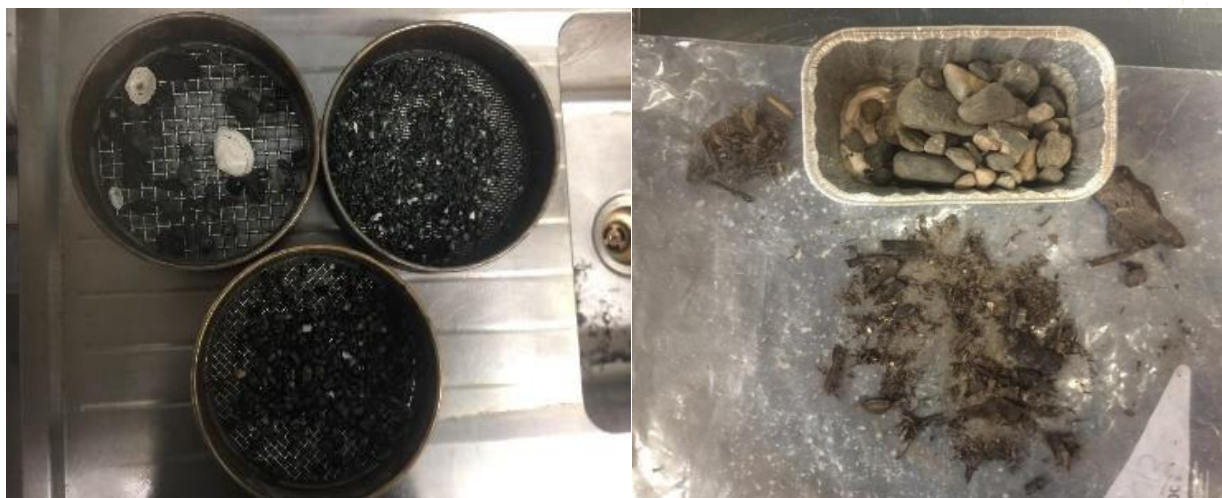
Figure 3. Left: samples were sorted through 9.5 mm, 4.75 mm, and 2.36 sieves to separate samples into four grain sizes. The finest grain sizes were washed through and collected in a pan. Right: the 9.5 mm and 4.75 mm grain sizes were hand-sorted into wood and bark, other organics, sediments, and shell components.
