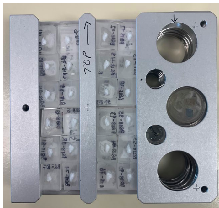
Figure 3. Otoliths of 24 Coho salmon loaded into the sample tray of an LSX-213 G2+ laser ablation system for analysis of trace elements. The signature of elements in the otolith provides insights into the migration history of the Coho to help identify whether that fish stayed resident in the Strait of Georgia, or migrated to the west coast. Photo by Micah Quindazzi
