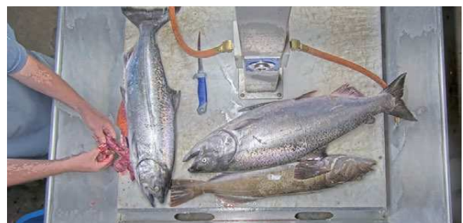
Figure 9: An example of the imagery captured while anglers are using the station to clean their catch. The recorded image provides enough resolution to identify the species and whether they were adipose fin clipped.
