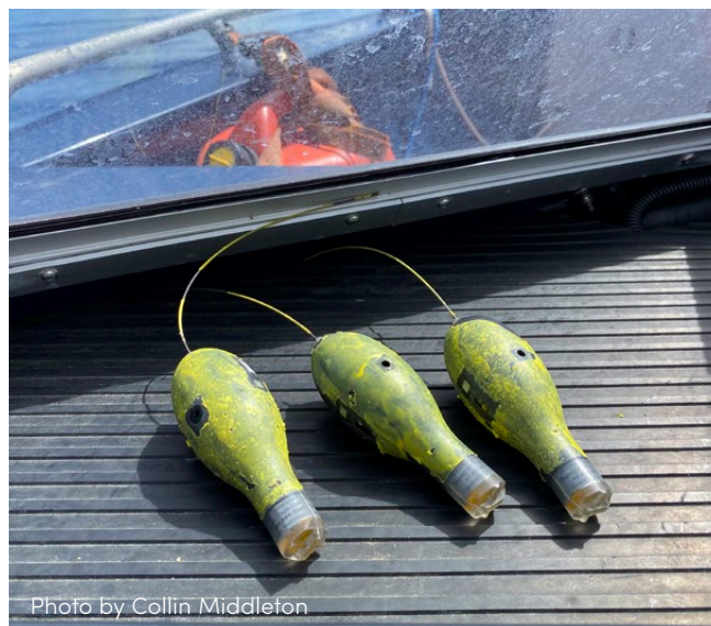
Figure 5: Recovered satellite tags. After a set period or after the fish dies, the satellite tags are designed to pop up to the surface and send out a signal that allows us to recover them. Once recovered we can download additional data and the tags can be recycled by the manufacturer for another deployment.
