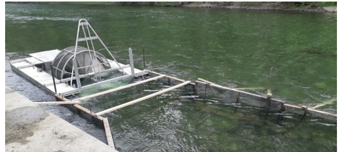
Figure 1: (Top) A'tlegay Fisheries Society Technicians sampling, from the mainstem Wolf Trap, outmigrating juvenile steelhead from the Quinsam River. (Bottom) The mainstem 8ft Rotary Screw Trap utilized for capturing salmon and steelhead in the Cowichan River.
