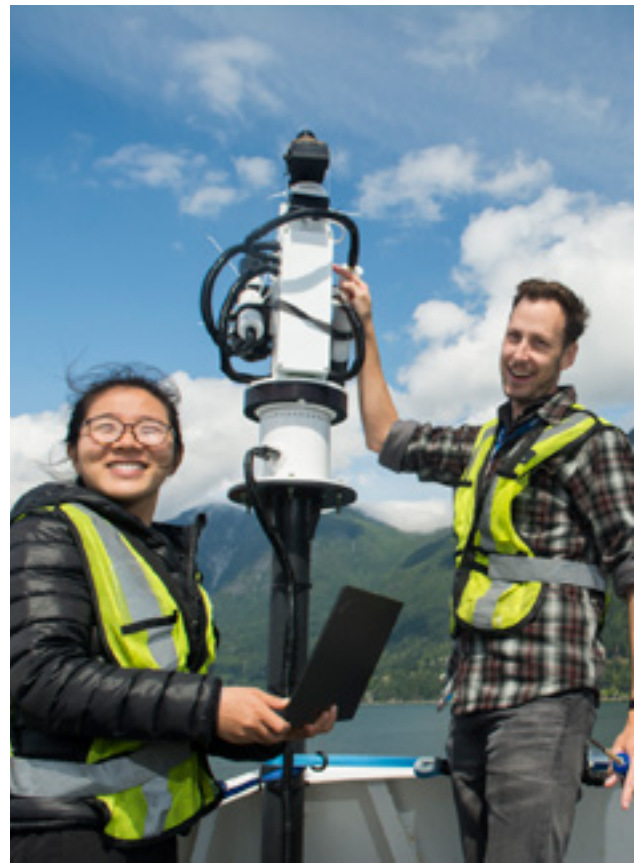
Figure 13. A hyperspectral above-water reflectance sensor used on BC Ferries. This sensor was used to validate satellite imagery, by gathering information on above-water reflectance. Photograph from Dr. Maycira Costa, UVic.
