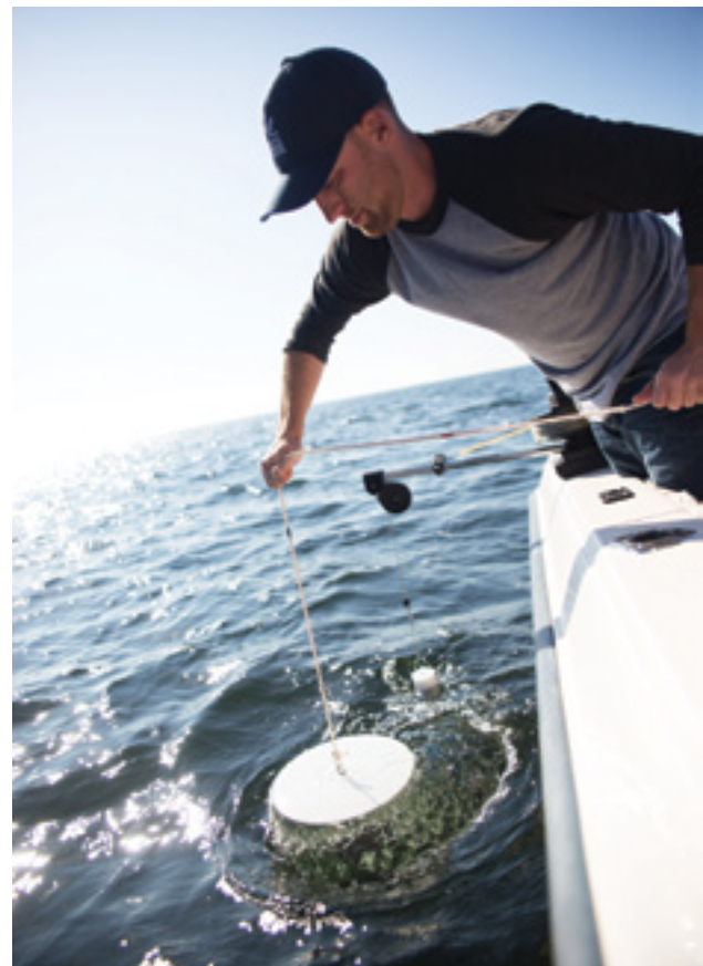
Figure 6. Steveston Citizen Scientist Billy McMillan lowers a secchi disk into the water to test for turbidity or water murkiness. Murkiness can block light and prevent plants that support salmon prey from growing.
