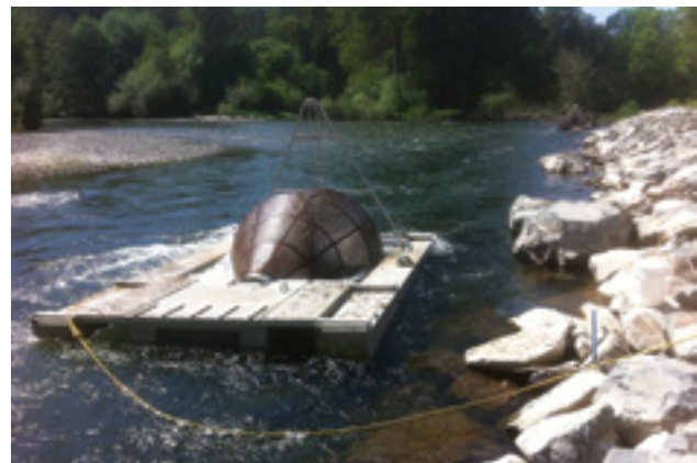
Figure 1. A Rotary Screw Trap (RST) is used to carry out mark-recapture studies of smolts and to estimate abundance of smolts.
