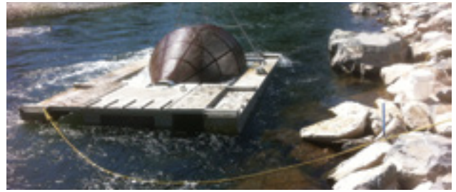
Figure 1. Rotary screw trap used to catch juvenile Chinook on Cowichan River
